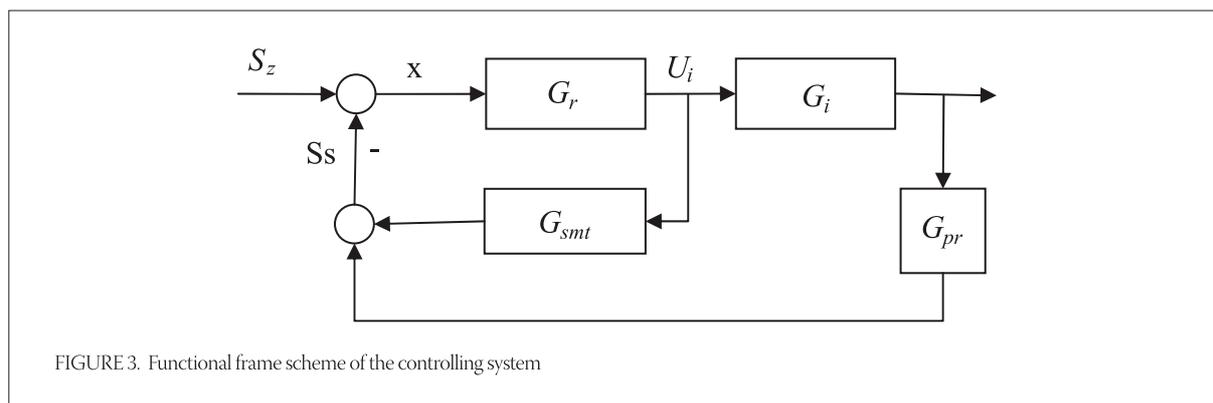
FIGURE 3. Functional frame scheme of the controlling system
